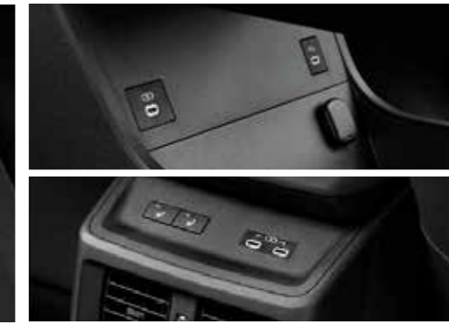
USB C Ports Two USB C ports, one at the front and one at the rear, allow convenient charging of smartphones and tablets etc., from anywhere in the vehicle.
