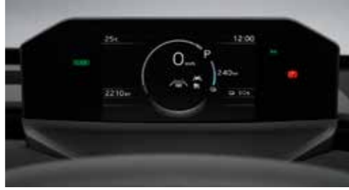
LCD Meter The top-mounted seven-inch TFT LCD meter features an advanced hoodless design. Positioned above the oval steering wheel, its layout minimises eye movement helping the driver to stay focused on the road.
