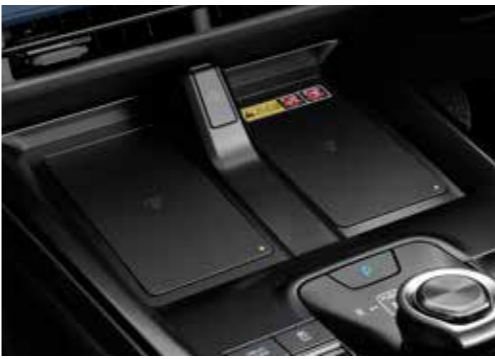
Wireless Charger A wireless charger for two smartphones, compatible with the Qi standard.
